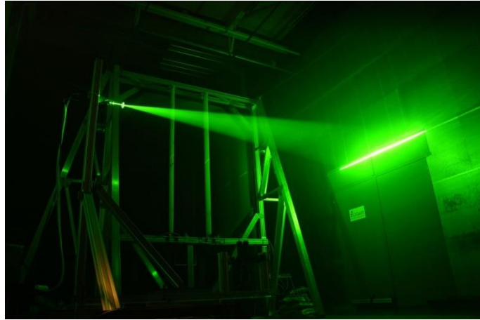
Figure 3: PIV light sheet/measurement plane
