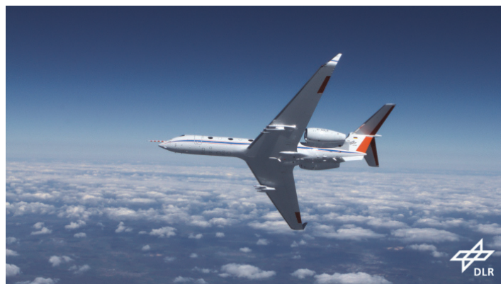
Figure 1: HALO during flight test with under wing stores.
