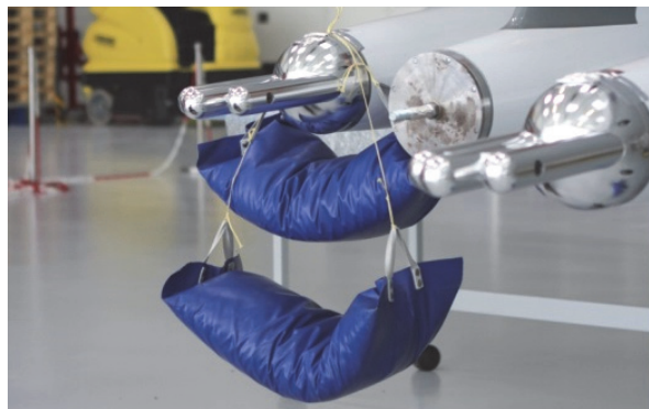
Figure 25: Strain gauge calibration of a PMS-carrier.
