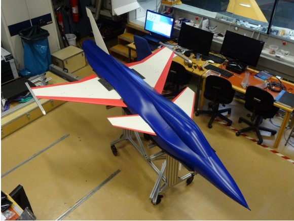
Figure 9: The generic fighter aeroelastic wind-tunnel model tested in summer of 2016.
