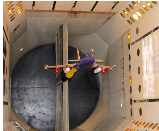
Figure 10: The generic fighter aeroelastic wind-tunnel model installed in the Transonic Dynamics Tunnel (TDT).
