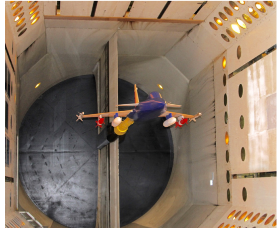
Figure 2: The generic fighter aeroelastic wind-tunnel model installed in the Transonic Dynamics Tunnel (TDT).
