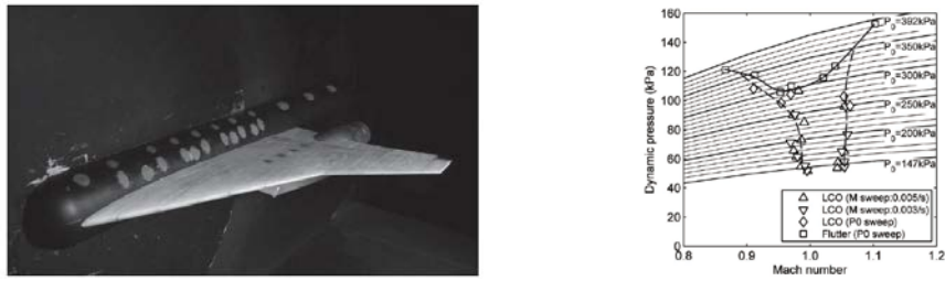
Figure 1: A wind tunnel model of jet powered experimental SST and its flutter boundary [1]
