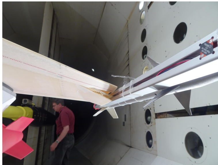
Figure 22: Wing tip damage.
