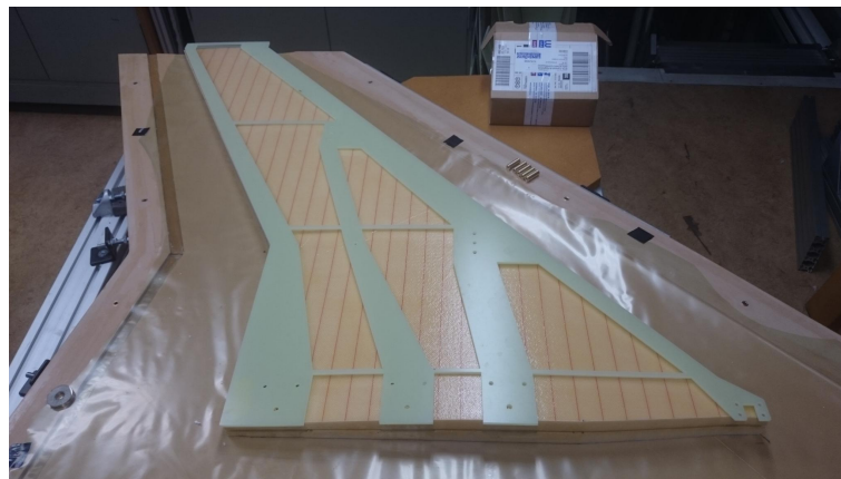
Figure 4: Internal wing skeleton structure.
