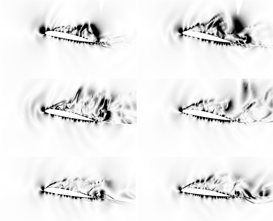
Figure 2: Visualization of flow patterns at six different times across stall by means of density gradients. Results obtained from SA-DDES calculations.
