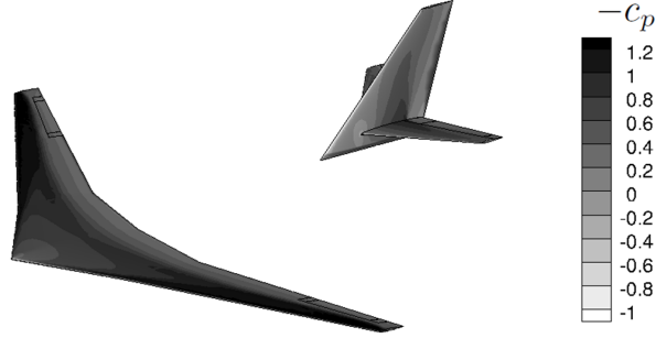
Figure 9: Inviscid wing empennage configuration. Steady pressure coefficient distribution at M_\infty = 0.84 and \alpha_s = 2 (deg).
