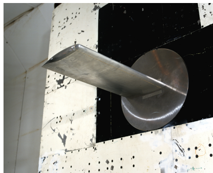
Figure 1: BSCW wing at NASA TDT wind tunnel section, Courtesy of NASA
