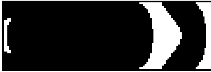
Figure 4: Final design for initial simplified plate wing model with a fundamental frequency constraint.
