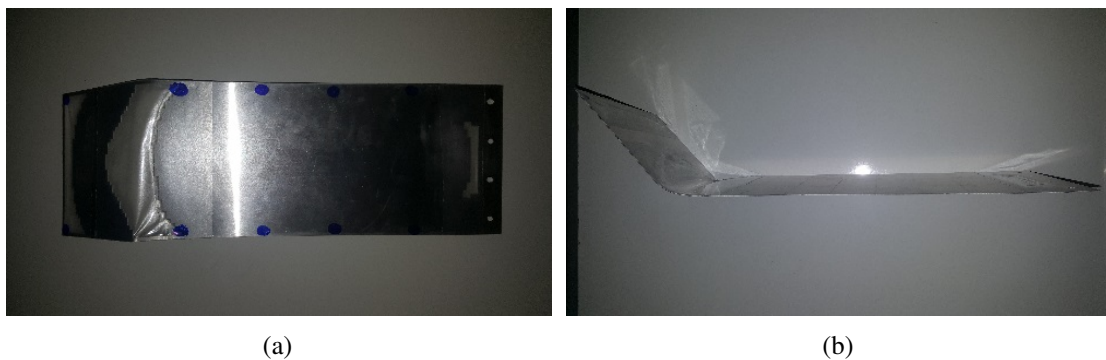
Figure 7: Wing failure with a frequency constraint.
