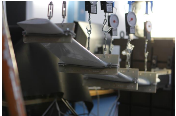
Figure 12: Static tests on Wing-1
