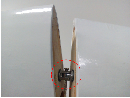
(a) Mechanical joint connection between two aircraft of the Experimental Multi-Body Aircraft
