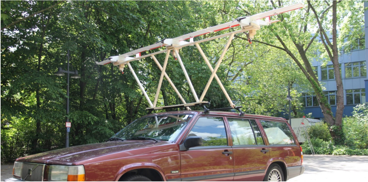
Figure 9: Take-off construction of the experimental Multi-Body aircraft installed on the top of a car
