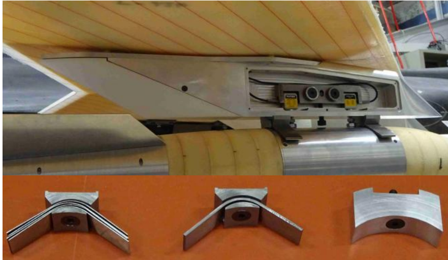
Figure 3: Model of pylon and sway brace. Load cells are measuring the preload.
