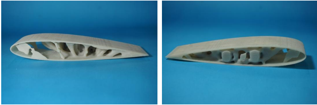
Figure 6: TO results manufactured by 3-D print.
