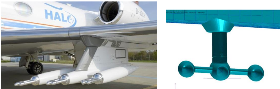
Figure 4. HALO PMS carrier and its simulation model
