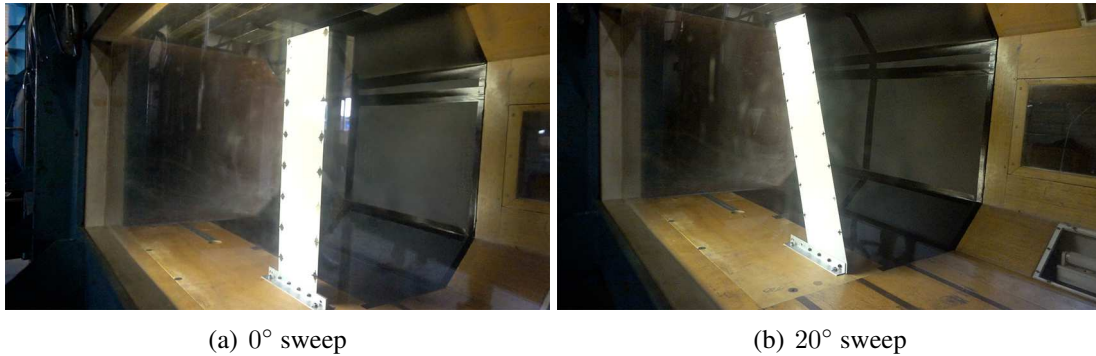
Figure 1: Two AR4 wings installed in the wind tunnel
