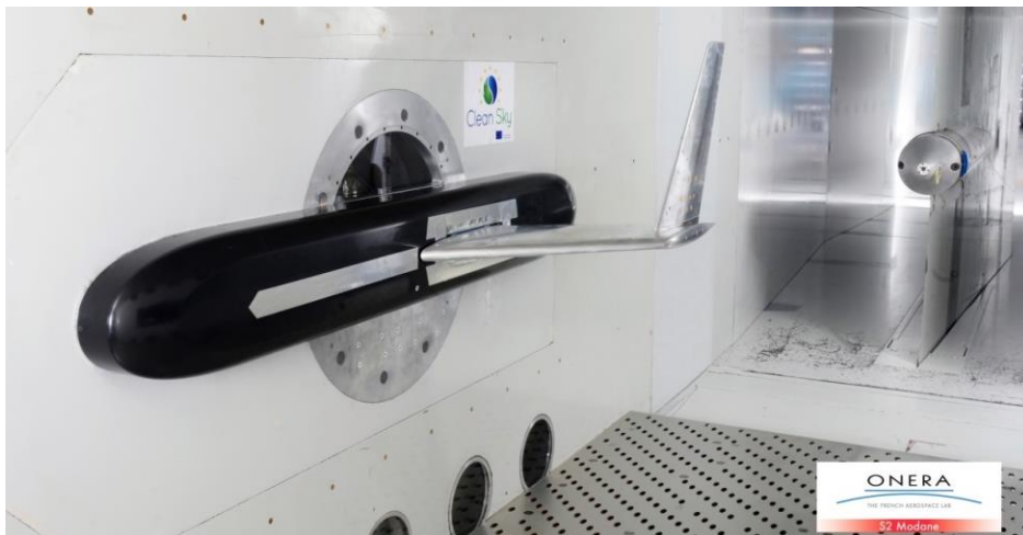
Figure 19: U-Tail flutter model in ONERA S2MA
