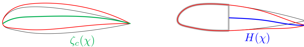
Figure 8: Types of morphing strategy: baseline geometry (black), camber morph (green) or trailing edge morph (blue) and resulting morphed geometry (red).
