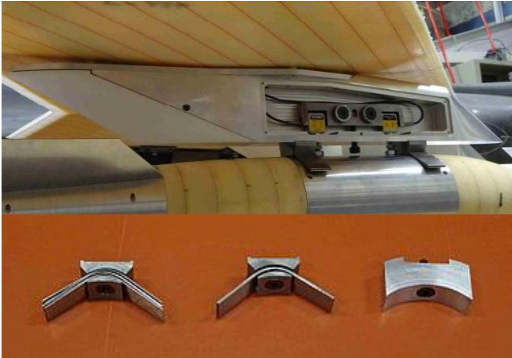
Figure 1 - Detail of pylon system (up) and sway brace options (down - multi-blade, single-blade, stiff).
