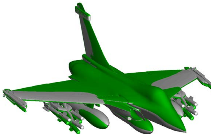
Figure 22: Rafale – Structural mode displacement (in green, scaled) and rigid shape (in grey)
