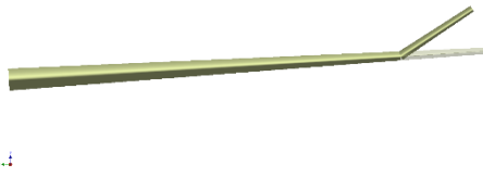
Figure 3: Front view showing positive fold angle for a hinge angle of 0^{\circ} .
