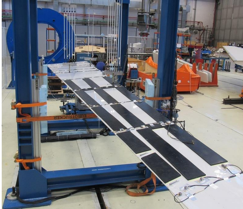
Figure 6: A/C elevator GVT with SBR damping layers.
