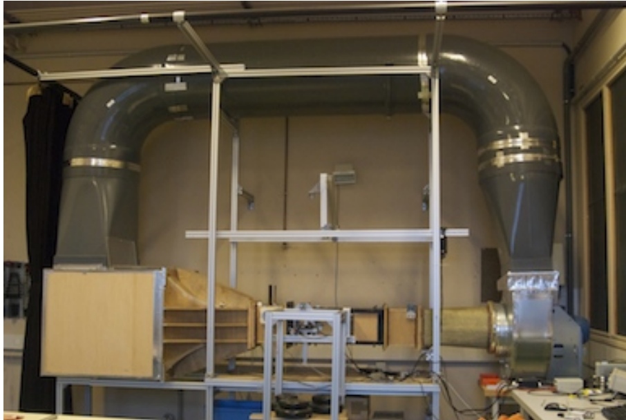
Figure 1: LadHyx Closed-loop subsonic wind tunnel
