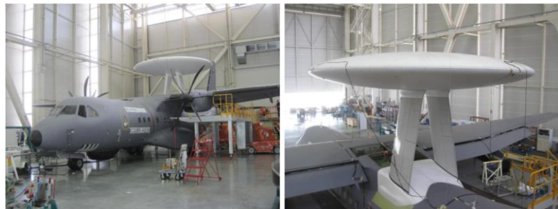
Figure 1: Images of the C295-AEW tap ground test to characterize the Dome normal modes
