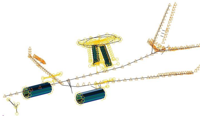
Figure 10: A330-AWACS condensed dynamic model
