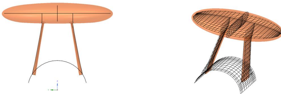
Figure 23: External geometry of the dome and struts (orange shaded contour) superimposed on the DLM lifting panels (black lines).
