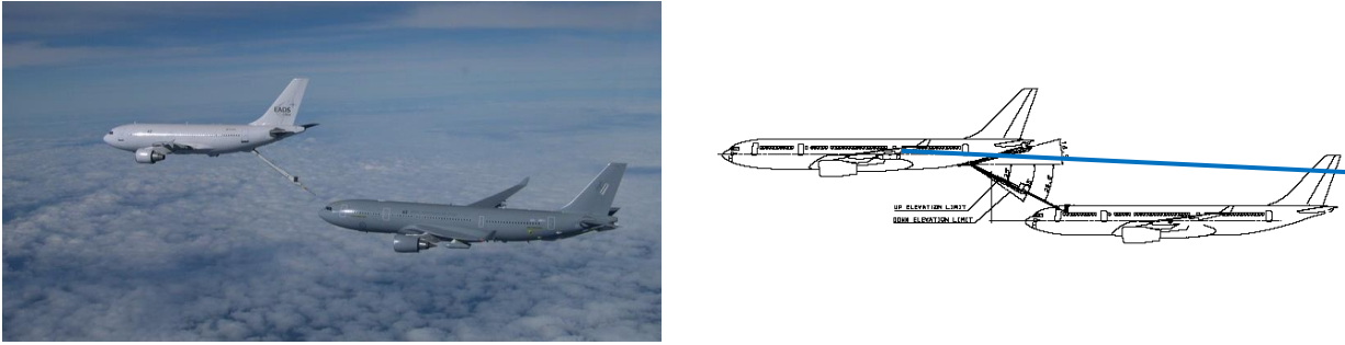
Figure 21: A330-MRTT being refueled by the A310-Demo (prototype to test the Aerial Refuelling Boom System)
