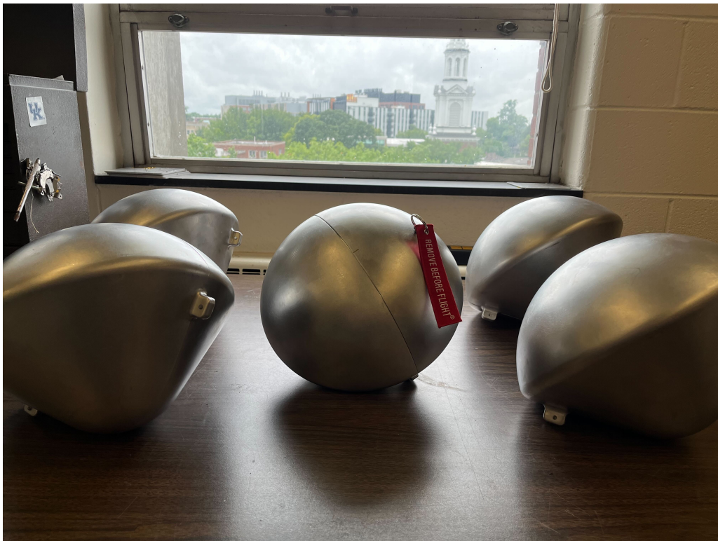
Fig 1. The five assembled KRUPS capsules of the KREPE-2 flight
