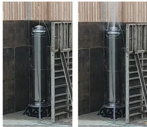
Figure 14: Motor case hydraulic burst test to validate margin of safety against Red Kite MEOP
