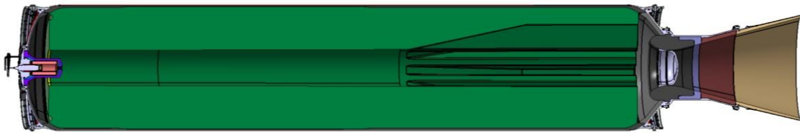
Figure 1: Red Kite Half Cut illustrating Finocyl Grain , Submerged Nozzle Design and Igniter Assembly [4]
