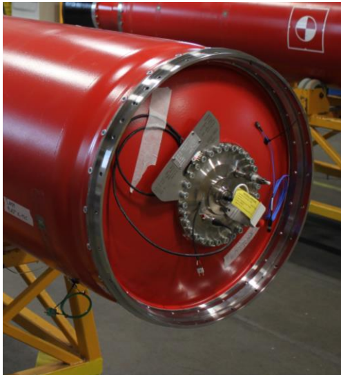
Figure 4: Front Mechanical Interface Joint and Igniter Assembly with SID and two pressure sensors installed
