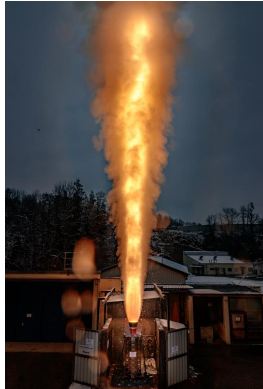
Figure 18: 2s overpressure test of full scale nozzle assembly to validate mechanical strength and thermal shock resilience
