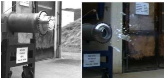
Figure 17: Burst test of nozzle seal
