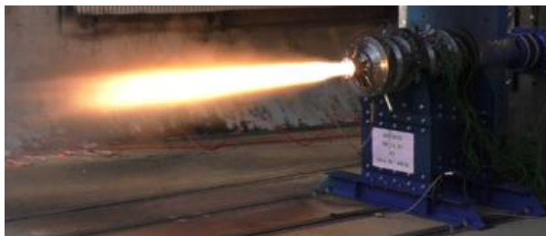
Figure 13: Subscale test firing to characterize nozzle material candidate
