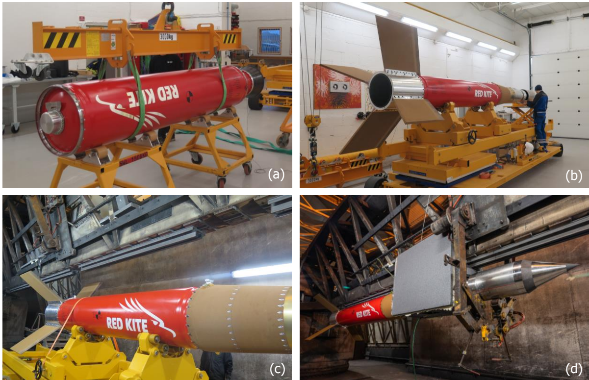
Fig 5. (a) motor as delivered, (b) vehicle fully assembled, (c) during loading, (d) during countdown
