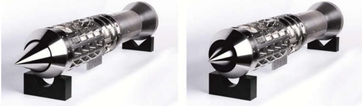
Figure 2. Wind tunnel model of the LK4 configuration of the ITEM-FK project
