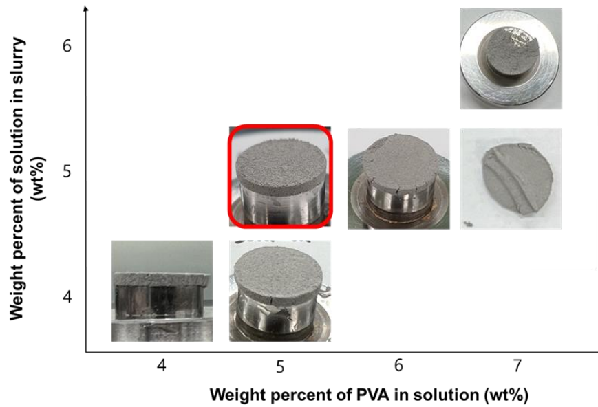
Fig. 4 Schematic diagram of the effect of PVA solution on metal slurry formability
