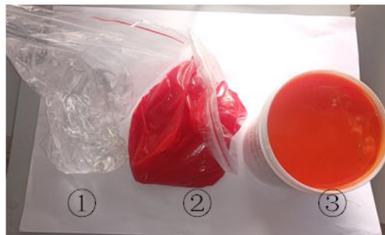
Fig 3. Domestic boric acid modified hydroxyl-terminated polysiloxane (PBDMS)
