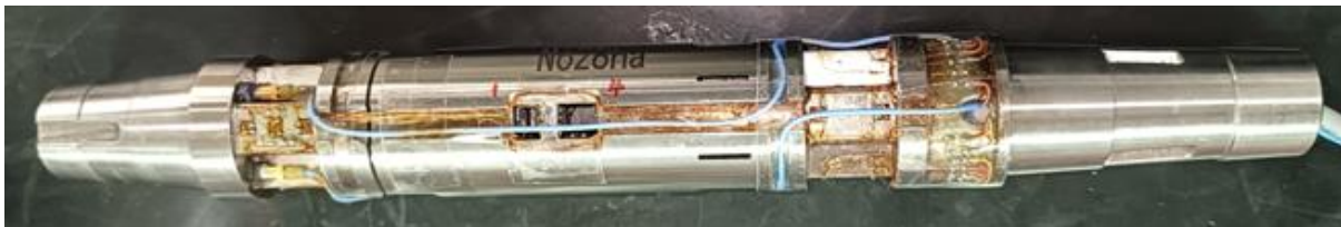
Fig 16. physical diagram of integrated design acceleration sensor and balance
