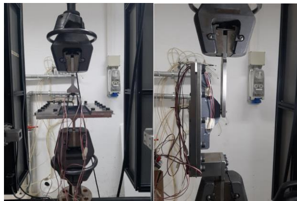
Fig 2. Tensile test and shear Y set-ups
