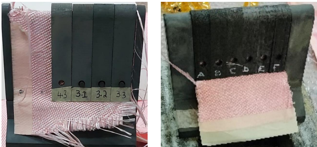
Fig 12. Nextel strip to insulate samples from graphite model holder
