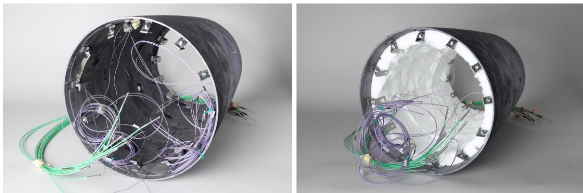
Fig. 10. CMC shell segment with installed sensors (left) and with installed high-temperature insulation (right).
