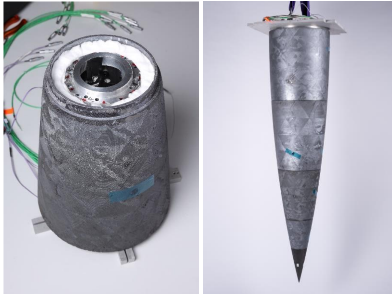
Fig. 11. STORT segment B before assembly (left) and the STORT forebody fully assembled (right).
