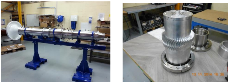
Fig 5. Hybrid air breathing propulsion – 200mm diameter preliminary demo and its 2 counter-rotating stages compressor
