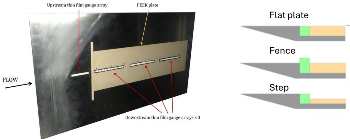
Fig 2. Experimental model with instrumentation annotated (left) example geometries of interest (not to scale) (right)
