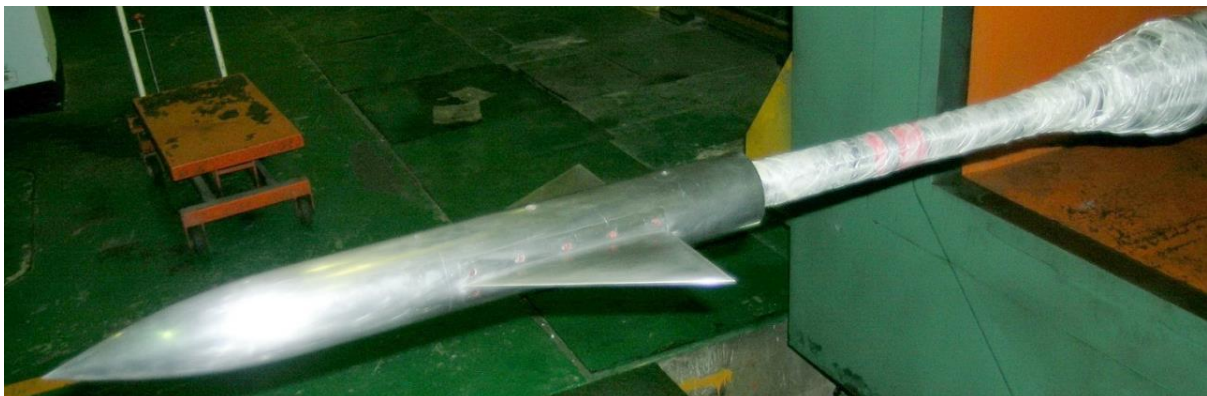
Fig.3 AGARD-B calibration model
