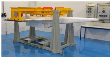
Fig 9. Mock-up and its handling tool (yellow part) on integration pad (in grey)
