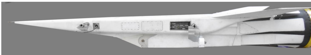
Fig 6. LEA vehicle and its Interface & Separation System
