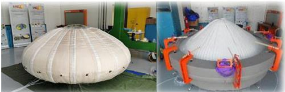
Fig 13. EFESTO-2: structural demonstrator and test-rig (vacuum-pool) at CIRA premises
