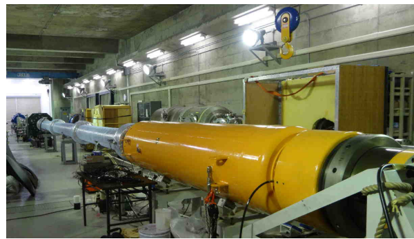
Fig 1. Schematic(top) and photos (bottom) of the free-piston driven expansion tube HEK-X
