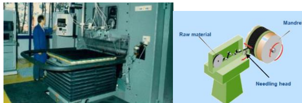
Figure 4: Genuine facility configurations for building flat Naxeco® preform (left) or axi-symmetrical parts (right)
