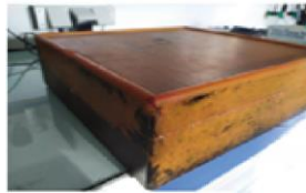
Figure 8: RTM and curing cycle validation for the Naxeco® resin material at small scale and simple plate (material aspect right after curing cycle)
