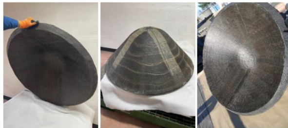
Figure 15: ESA PREHEAD's 1m base diameter heat shield 3D fibrous preform demonstrator after phenolic resin transfer
