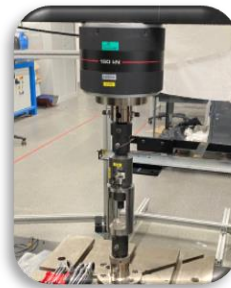
Figure 9: Characterization of mechanical properties and assembling joints for the Naxeco® Resin
