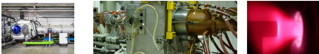
Figure 10: DLR L3K arc heater (credit DLR, left), ArianeGroup plasma torch (center), PWK1 (credit IRS, right), used to investigate the thermos-erosive behavior of the materials
