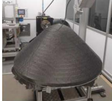
Figure 14: ESA PREHEAD's 1m base diameter heat shield 3D fibrous preform demonstrator after needling consolidation
