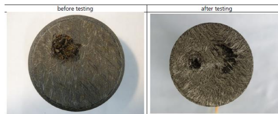
Figure 12: Comparison of pre-damaged L3K sample with HVI of the exposed surface before the plasma exposure (left) and after plasma exposure (right)
