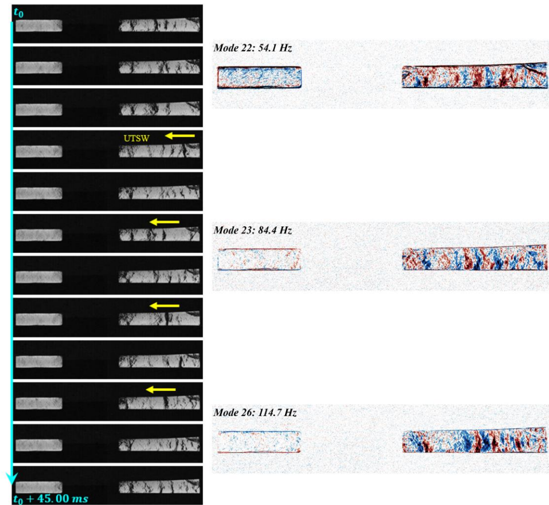
Fig 11. Isolator-scrumjet combustor results in case 5: (Left) Instantaneous snapshots of shock train and UTSW (Right) sub-mode
