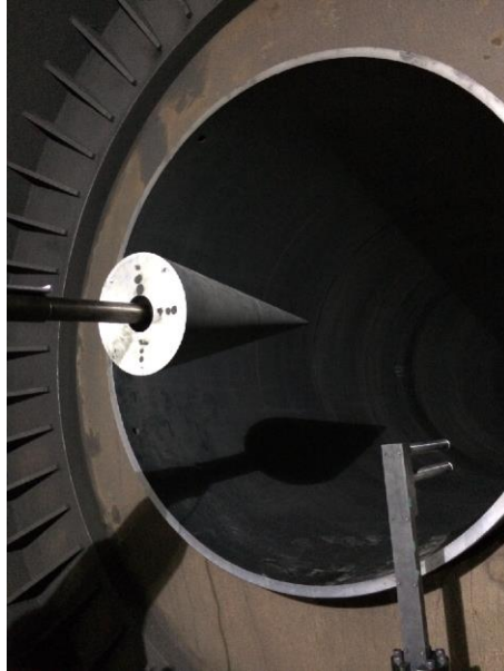
Fig 12. Validation of axial force processed by CNN frequency-domain model. Force test in JF-12 shock tunnel.
