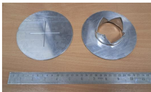
Fig 3. Primary Diaphragm (Left: Before rupture, Right: After rupture)
