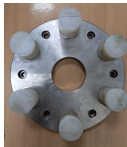
Fig 5. Teflon buffer after a test run
