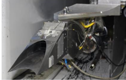
Fig 6. Test model of the inward-turning TBCC inlet in the wind tunnel.
