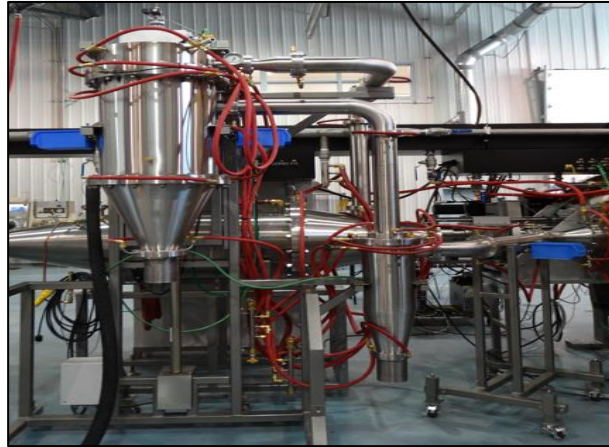
Fig 17. Particle trap and filtration system with an S duct to deviate the powder to the filtration system.
