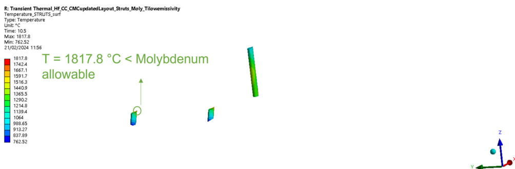
Fig 12. Molybdenum struts thermal result.
