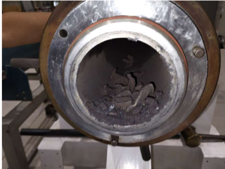
Fig. 7 Diaphragm debris found at the end of the Driven Tube.
