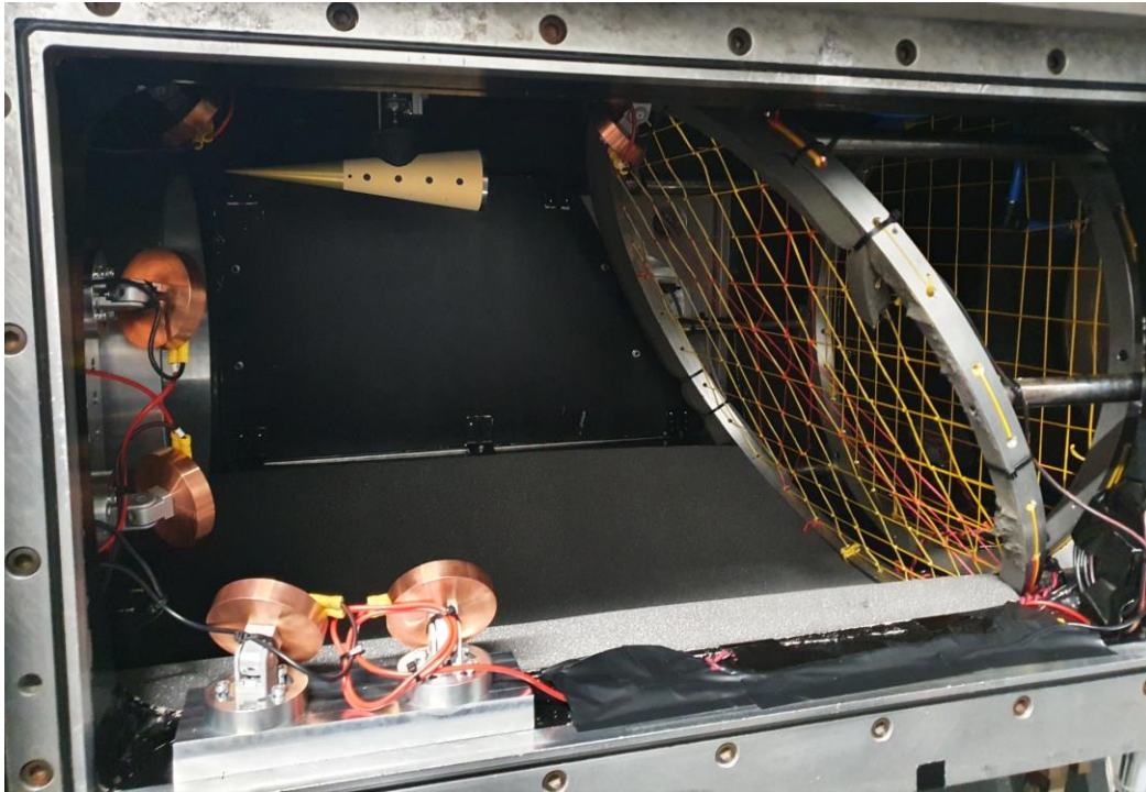
Fig. 7 PSP-coated free-flight cone model mounted in the HDT test section prior to a test.
