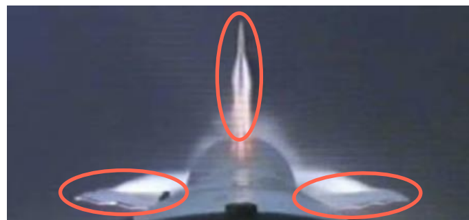
Fig 2. SHEFEX-1 - 2 nd -Stage fins during re-entry at approx. Ma=6-7 at H=20\text{km} altitude – Buckling of the metallic leading edges [1]
