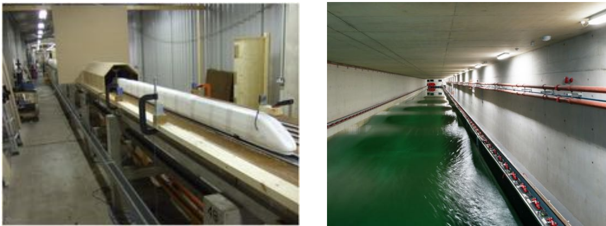
Fig 3. The 1/25^{th} -scale, 150 m-long catapult-driven TRAIN rig at Birmingham University with a 50 m test section (left) and the 138 m-long towing and wave tank at the University of Southampton with maximum carriage speed of 10 m/s (right)
